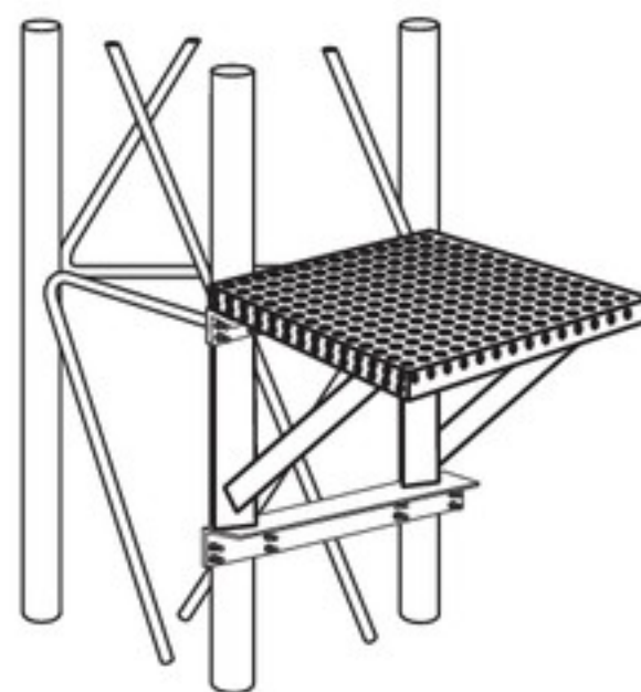
WORK PLATFORM WPCC65 SNAPS INTO PLACE AT ANY LEVEL. NO BOLTS REQUIRED.
