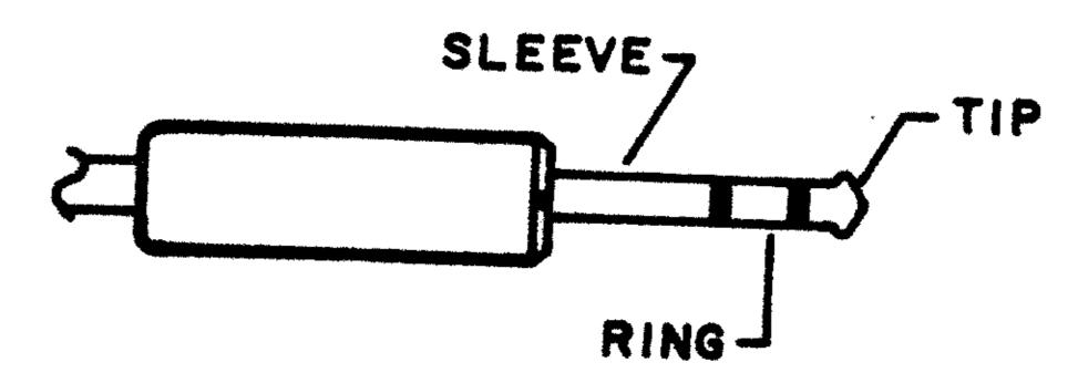
Figure 1-2. Tip-Ring-Sleeve Plug Outline Drawing.
