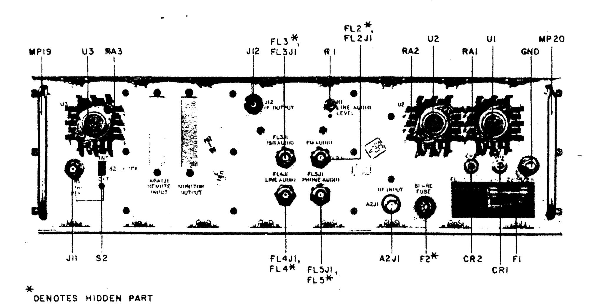
Figure 7-1. WJ-8716 Main Chassis Rear Panel View Location of Components
