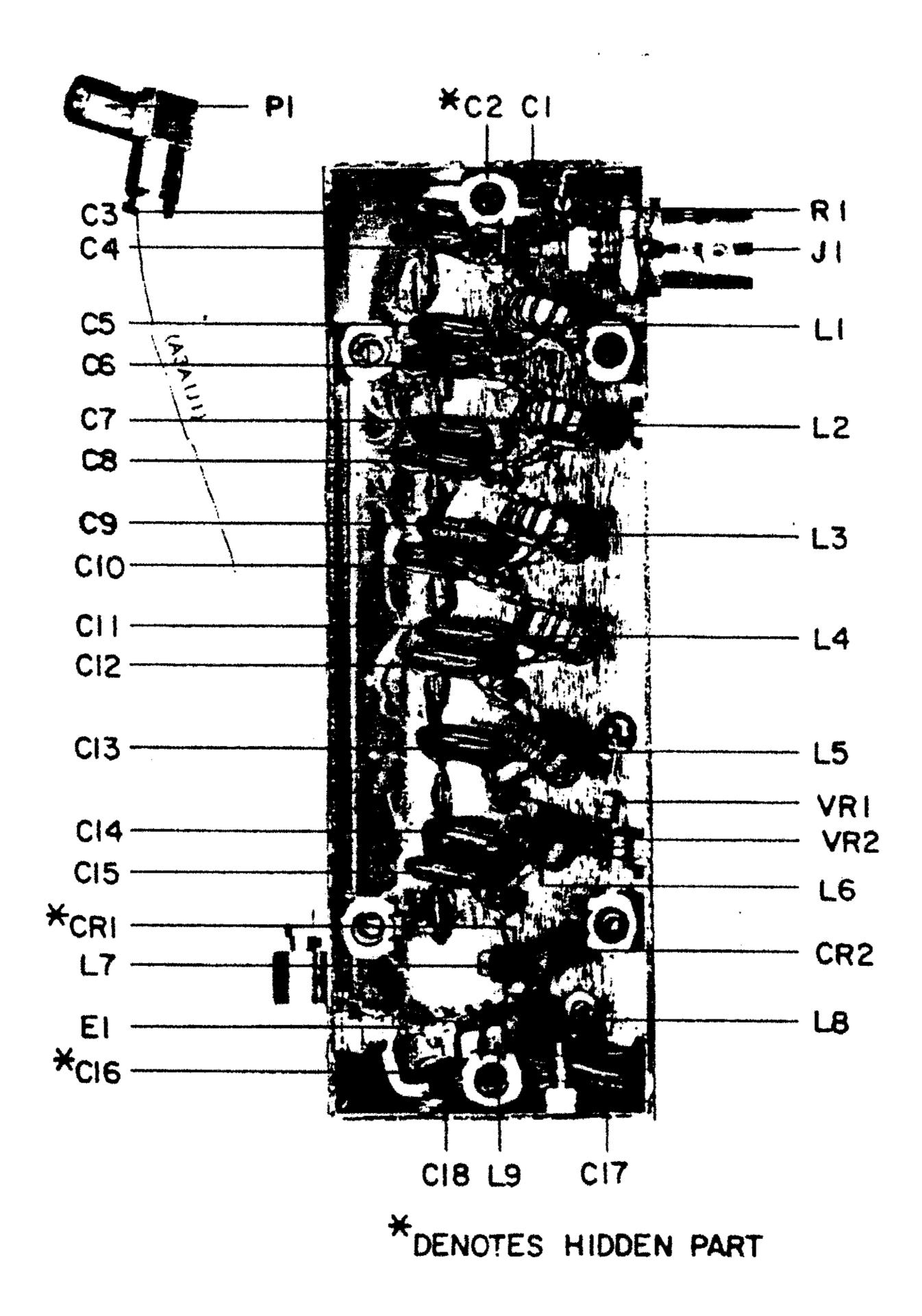
Figure 7-2. Type 795010 RF Filter, Location of Components
