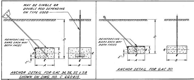
89 NOTE: QUE TO VARIABLES INVOLVED IN ROOF AND OTHER INSTALLATIONS, IT SHALL BE THE CUSTOMER'S OR INSTALLER'S RESPONSIBILITY TO PROVIDE STRUCTURALLY ADEQUATE SUPPORTS FOR PIER & ANCHOR CONVECTIONS. IT MAY ALSO BE NECESSARY FOR THE CUSTOMER OR INSTALLER TO SECURE THE SERVICE OF A LOCAL ENGINEER TO DETERMINE THAT INSTALLATION COMPLIES WITH LOCAL BUILDING CODES.
