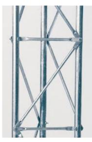
As with all ROHN products, Rigid Tube Towers are Hot Dip Galvanized after fabrication to assure years of corrosion free use. In this process, each section of the tower is totally immersed in molten zinc, bonding 2 ounces of the zinc to every square foot of steel. Hot Dip Galvanizing protects all surfaces, inside and out, against rust and corrosion while providing an attractive finish.
